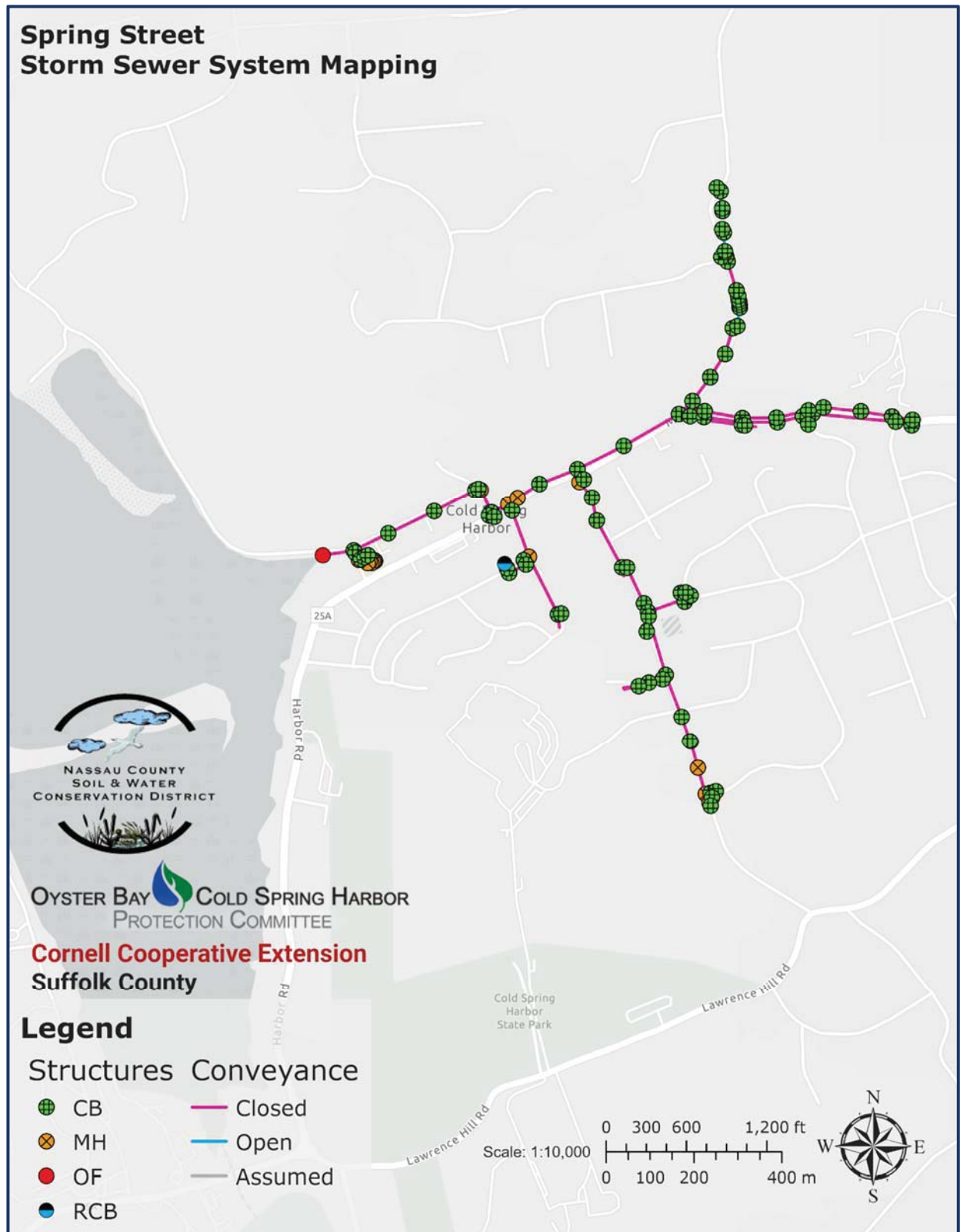
Figure 6. Spring Street Outfall # 273 storm sewer system conveyance mapping.
